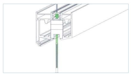
Using one of the 5.0 x 45mm screws, secure the middle restrictor block as shown.
