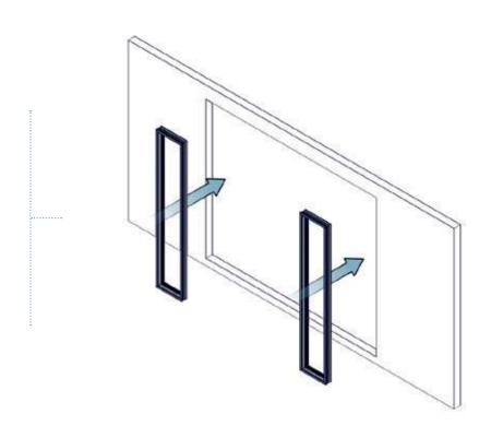
Ensure the remaining aperture is 6mm wider than the overall door set width
