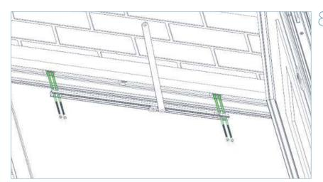
Now place the slider casing back into the top track at your marked position, and secure the last 4 restrictor blocks through the slider casing using the 5.0 x 60mm screws as shown. It may help to disconnect the sash pivot at this point for ease of installation. Once the screws have been fitted reconnect the sash pivot. Check the door for proper operation.
