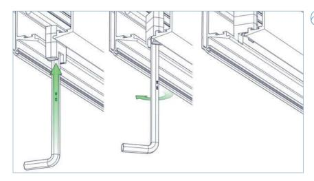
Insert four of the restrictor blocks positioned at the points you have marked on the top track. Do this by using an 8mm Allen key to insert the block into the track and twisting 90° clockwise to lock it in to place. The 5th restrictor block is then inserted half way between the other blocks.
