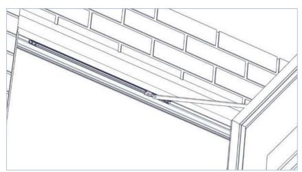
Insert the slider casing into the top track making sure it is still connected to the sash pivot, it should only fit in one position. Then, using a non-permanent method, mark the positions of the four screw holes in the slider casing, then move the slider casing out of the way.
