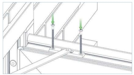
Fit the sash pivot to the top of the door, 60mm from the end of the black polyamide strip on the hinge side using two of the 5.0 x 45mm screws provided. The pivot should be fitted so that it butts up to the edge of the polyamide closest to inside of the door.
