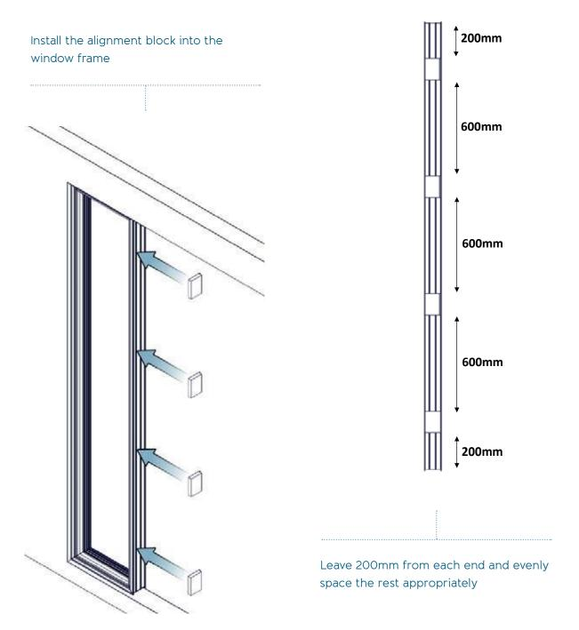
Drill, countersink and fix alignment blocks
