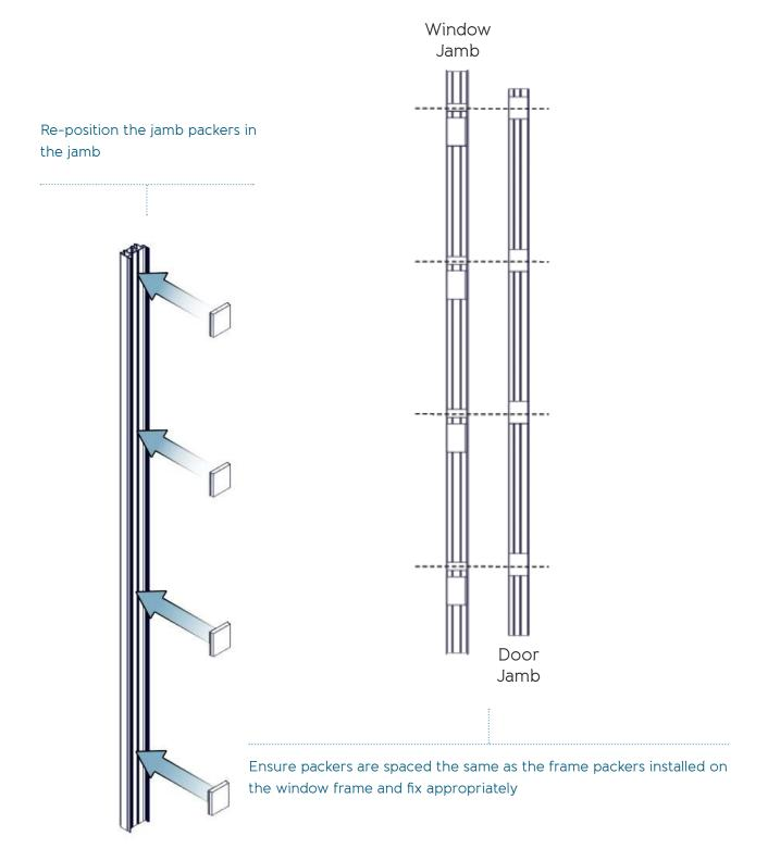
Position the door frame into the aperture and pack/ clamp accordingly
